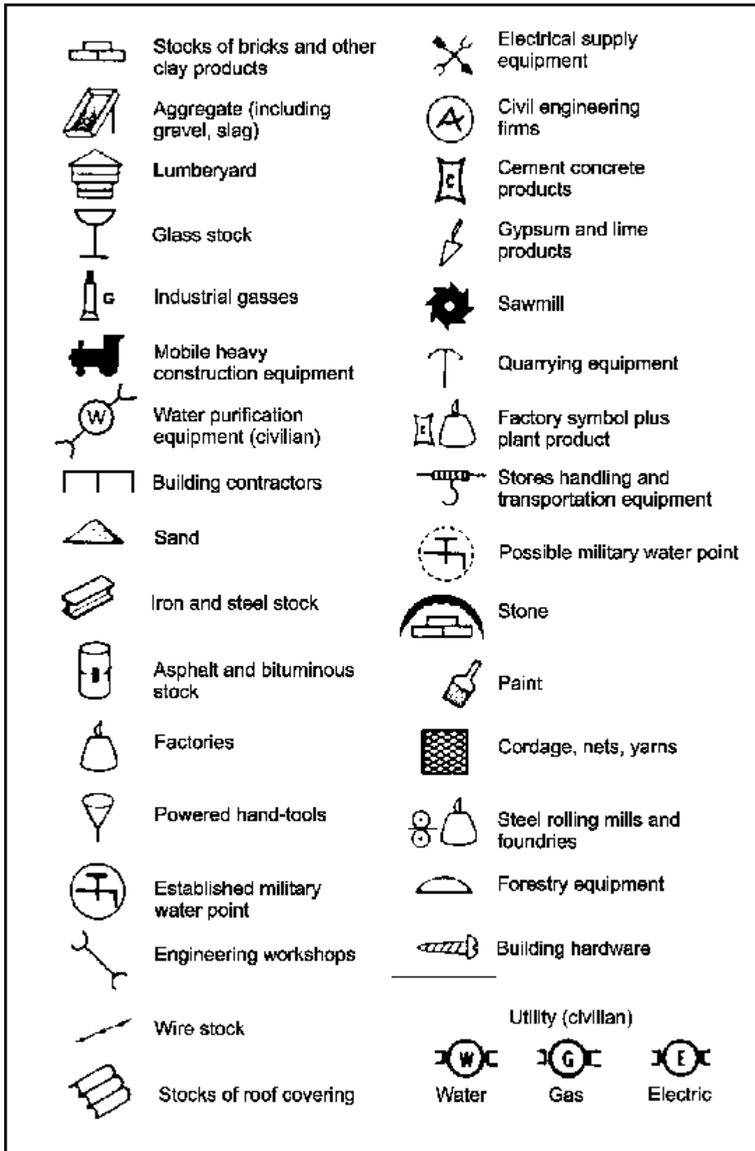
Figure 9-3. Material, facility, equipment, and service symbols.
